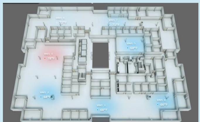
The GUI offers easily interpretable information starting at the 3000-foot view. For example, from this heat-map view, the end user is able to quickly determine any problem units via a visual temperature indication.
