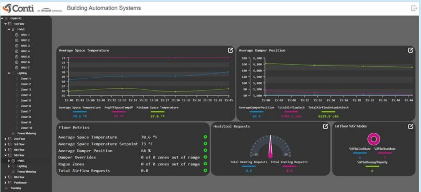
Floor-level metrics allow a secondary evaluation of floor-level conditions, easily identifying any deficiencies in floor-level units or the upstream units serving the floor. From one graphical page, the end user can determine mode, operation and operator overrides that could negatively influence the space.
