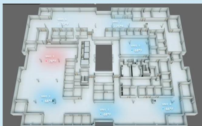
The GUI offers easily interpretable information starting at the 3000-foot view. For example, from this heat-map view, the end user is able to quickly determine any problem units via a visual temperature indication.
