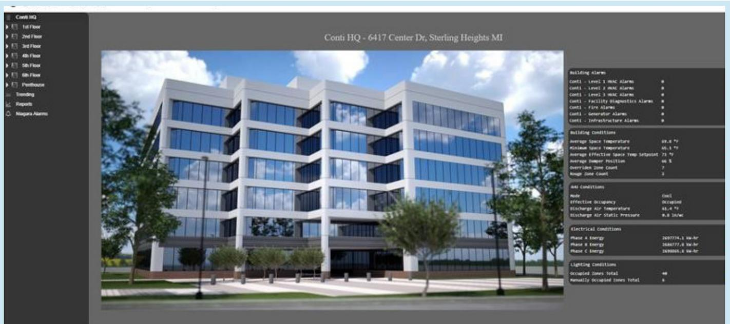
Example of a Conti-developed home screen for a large building. The graphical user interface (GUI) needs to provide for easy navigation from the portfolio-level, to floor-level, down to pieces of equipment and even VAVs. Visualizations are designed for easy, unambiguous interpretation to facilitate quick reaction and resolution of alarms.
